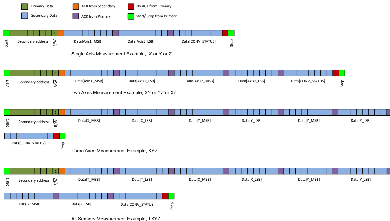
Figure 7-11. 1-Byte I 2 C Read Command for 16-Bit Data With CRC Disabled, CRC_EN = 0b
